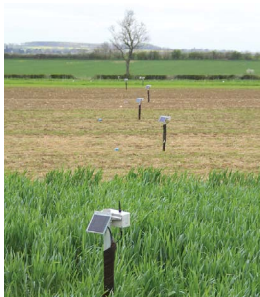
Soil moisture probes
